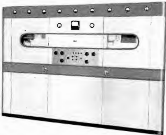
Gates 10,000 watt amplifier, 11' wide, 84" high and 50" deep. Employs four 892R audio amplifier tubes in the output stage.
