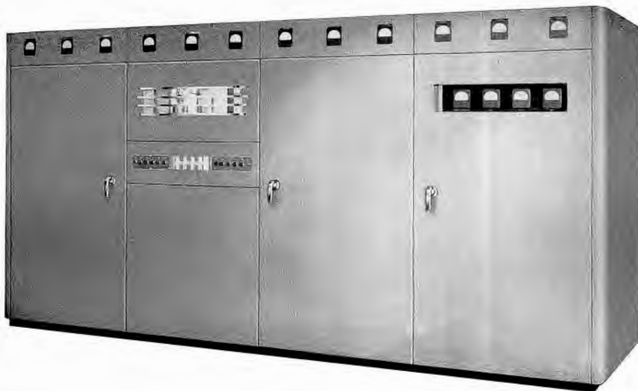
The Transmitter With Phasor
