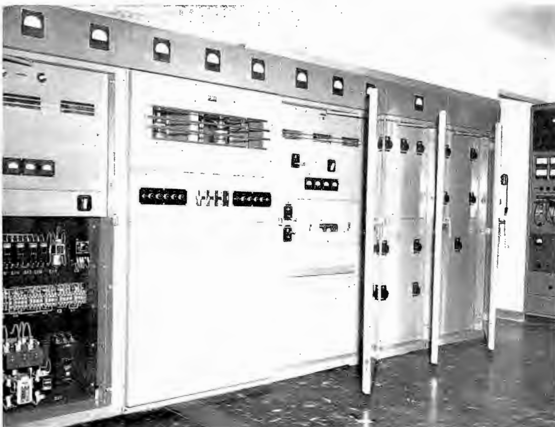
Below—Gates BC-5B 5000 watt equipment with five tower phasing equipment in matching cabinet at WENE, Endicott, N. Y.
