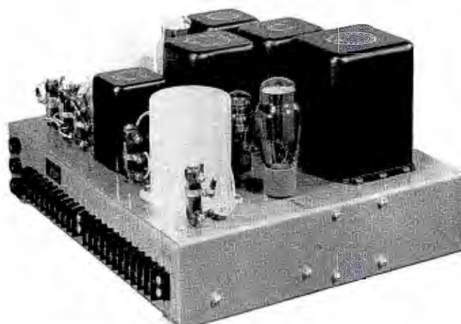
Above, left, the low voltage power supply deck. Right, the main high voltage supply delivering 2300 volts to power amplifiers and modulators.
