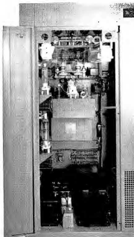
These two rear views of the HF1 transmitter picture the left section of radio frequency portion. The engineer will note the symmetrical design which assures perfect circuit balance, necessary for high efficiency and stability.
